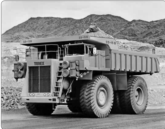
Terex 33-15B hauler, 170 tons capacity.
