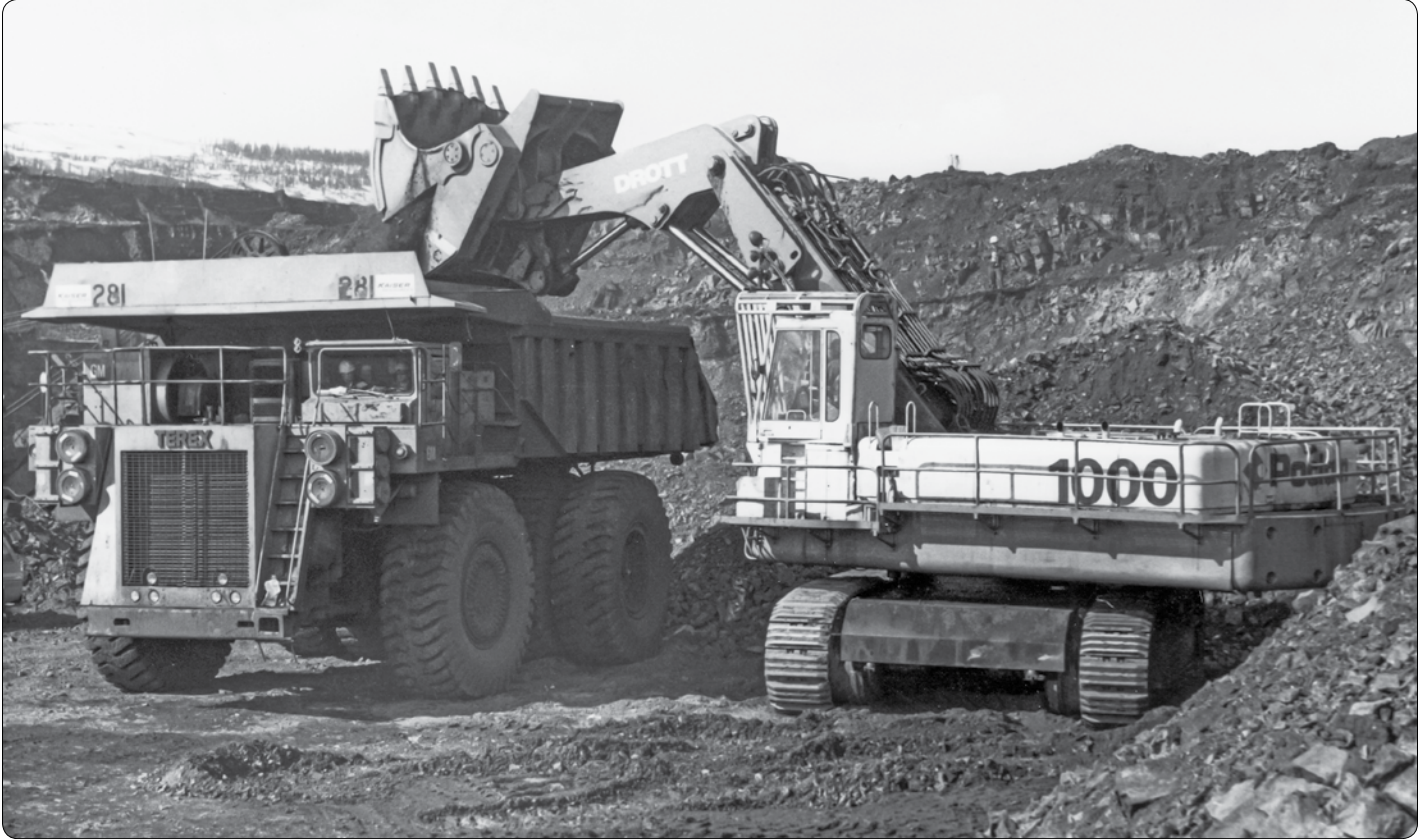
A 33-15B receives a load from a Poclair 1000CK at the Balmer Mine, Sparwood, British Columbia, in 1978. The Drott name on the boom stems from both brands being owned by Tenneco.
